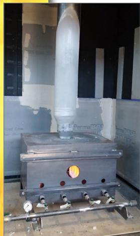
Testing a wood-burning stove heat shield.
