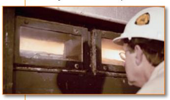
"tunnel test," it checks the "Surface Burning Characteristics of Building Materials." It was introduced in the early 1920s to evaluate "white wash" coatings. Currently, virtually all materials in buildings and other structures that require acceptance from national code bodies undergo the tunnel test. Typically, results are designated by code bodies as class A, B and C.
