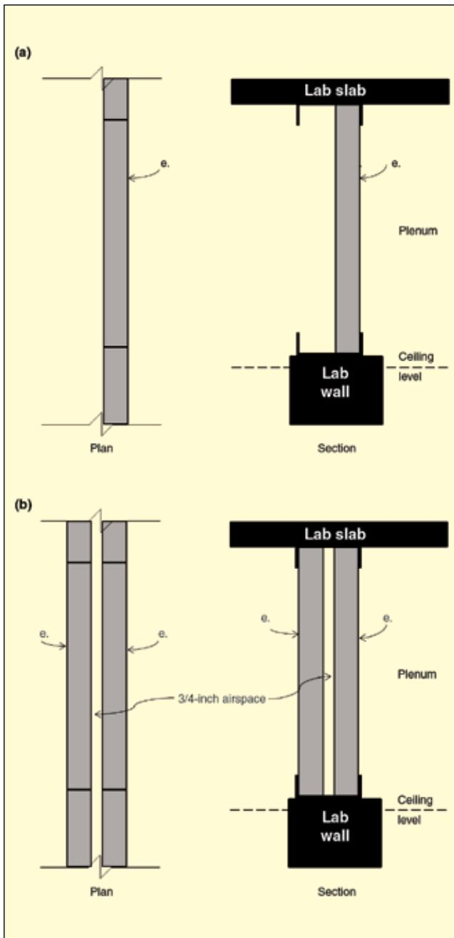
Figure 7. (a) Stone wool plenum barriers (insulation type e in materials list) one layer only (b) two layers separated by a 3/4-inch air space.
