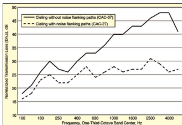
Figure 1. Noise flanking paths caused by common elements penetrating ceiling system can result in significant degradation to isolating capacity of ceiling system.<sup>2</sup>
